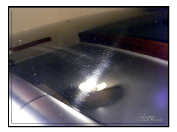
As you can see, the paint has suffered significant damage over the past few years. It is incredibly difficult to capture on film the extent of the swirling on the paint. It almost looks like it has been scrubbed, top to bottom, with steel wool! Of more concern, however, were the much deeper scratches (that look to have been inflicted by the family dog jumping up against the doors), dings, and even paint transfer from various parking 'incidents'.
