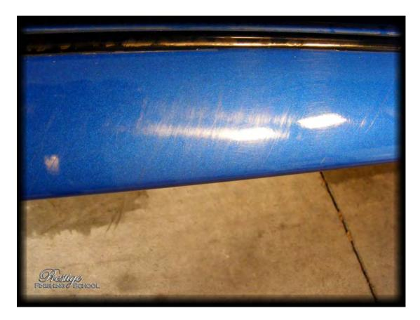
And again, notoriously difficult to convince the camera to focus on the defects, but you can plainly see the damage caused by footwear being scraped on the sill. This shot of the spoiler was snapped out in the sun prior to the wash.
