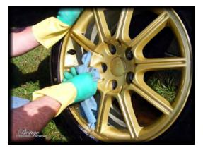
They were then treated to a top-up coat of Poorboy's Wheel Sealant which serves to protect the bare alloy of the inside rim and helps to prevent etching, pitting and oxidization.
