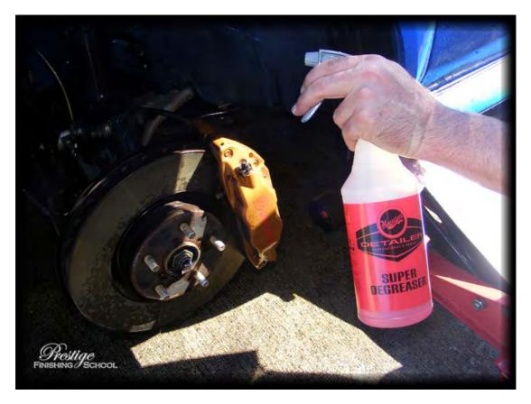
It also allows us to ensure that the brake calipers are completely clean.
