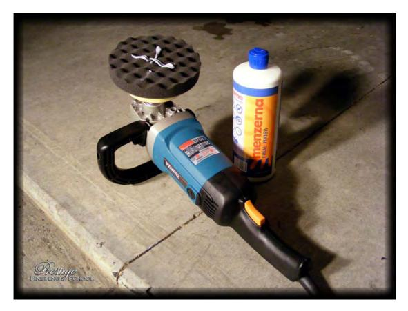
The machine is fitted out with a 3M rotary backing plate and 3M polishing pad. Given the German subject, we opted for Menzerna polishes – starting off with the least aggressive 85RD
