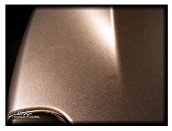
This was cleaned up by hand with more of the 3M polish on a microfibre work cloth.
