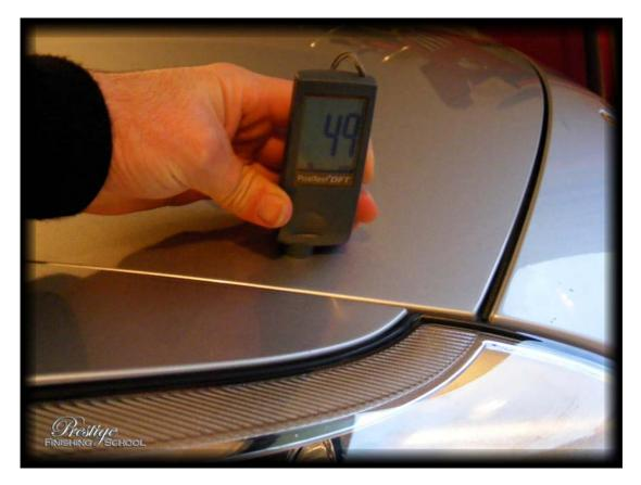
Undertaking any corrective action on this level of paint with aggressive compounds or polishes would run a significant risk of "striking through" the protective clear coat altogether. Such a misstep would necessitate a complete re-spray of the panel, so we always check every panel before, during and after any of our details.
