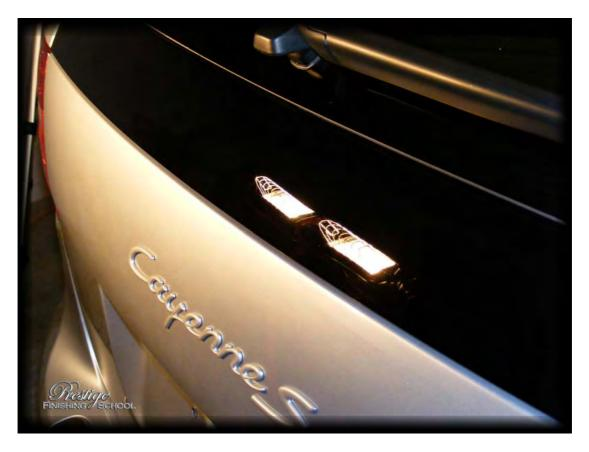
The scratches at the base of the tailgate were not so easily moved. These required a slightly more aggressive treatment, but not significant cutting or compounding. In this case, 3M's "Extra Fine Polish" on a new 3M polishing pad did the trick.
